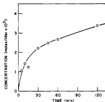
**Figure 2.** Total hydroperoxide yield vs. time in the photolysis of methylcyclohexane: oxygen; mercury resonance lamp; no filter.
