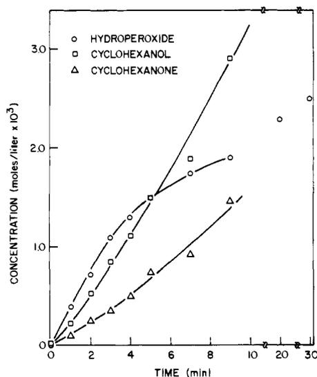
**Figure 1.** Product concentration vs. time in the photolysis of cyclohexane: oxygen; mercury resonance lamp; no filter.
